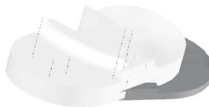
Figure 23 – The second constraint and the model obtained using the Mate command
