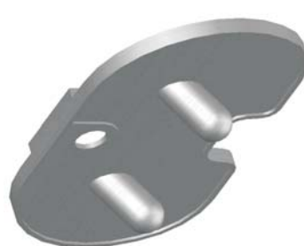
Figure 11 – The final model of the tibial metallic component
