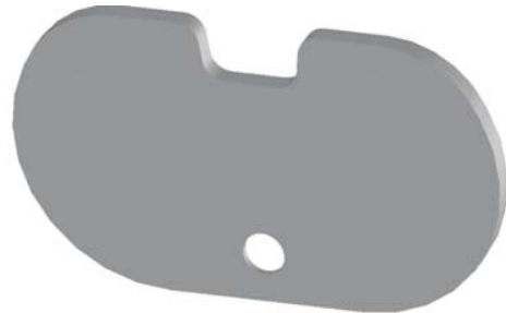
Figure 7 – The obtained model after the Cut-Extrude command
