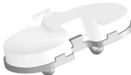
Figure 24 – The final model of the tibial knee prosthesis
